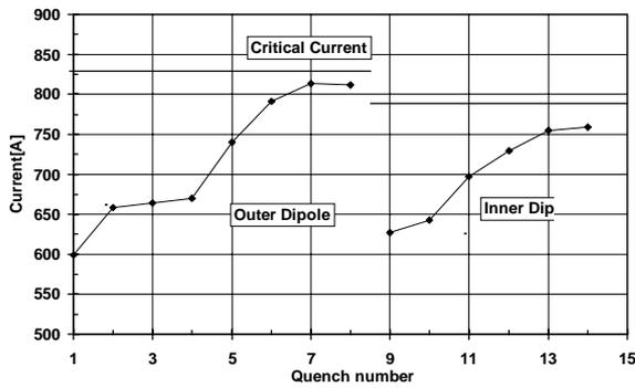
Figure 1: Inner and outer dipole training at 4.3K
