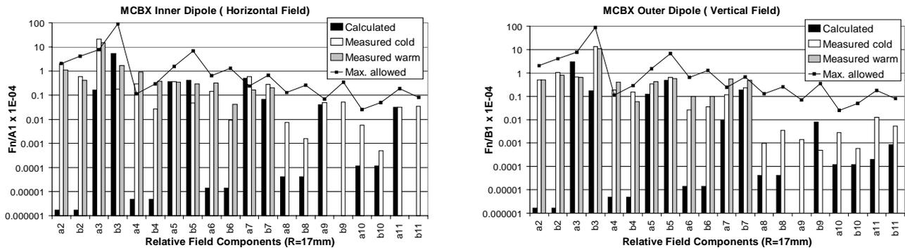
Figure 4: Relative field errors of MCBX inner and outer dipoles at nominal current.
