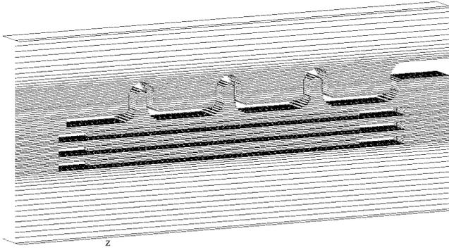
Figure 6: Lower half of a Snake-Coupler with a 3-cell flat field resonator ( $Q_{ext} \approx 1000$ ).
