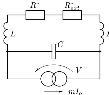
Figure 1: Equivalent circuit for a beam driven rf cavity resonator
