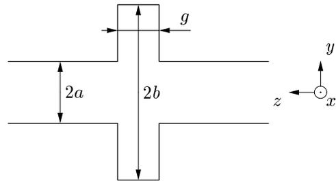
Figure 4: Two-dimensional single cell resonator for 91.39 GHz, optimized for maximum shunt impedance for a  $\beta = 0.302$  beam:  $a = 0.3\text{mm}$ ,  $b = 0.925\text{mm}$ ,  $g = 0.4\text{mm}$ ,  $Q = 1250$ ,  $R' = 520\Omega\text{cm}$ .
