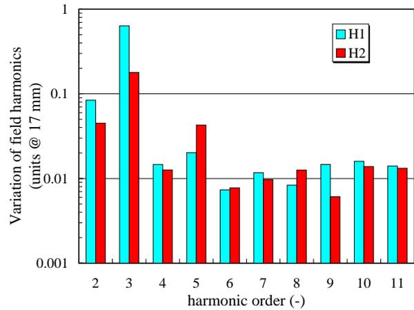
Figure 4. Maximum range of variation in the harmonics throughout the testing period for the H1 and H2 dipoles.
