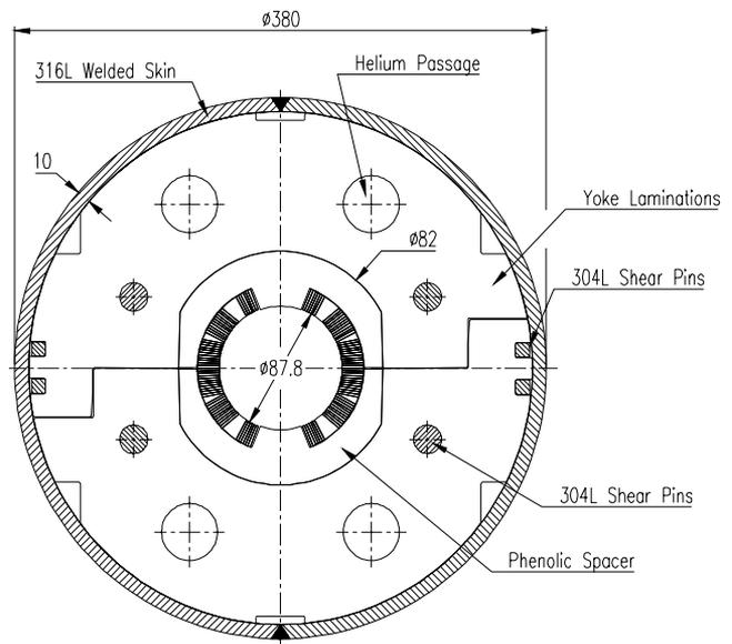
Fig. 1: Cross section of MBXSM type model.
