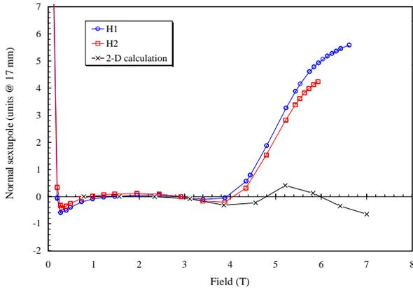
Figure 3. Measured and computed sextupole for H1 and H2 dipoles. Measured values have been shifted by the amount reported in Table 2 to remove the geometric sextupole and ease the comparison.
