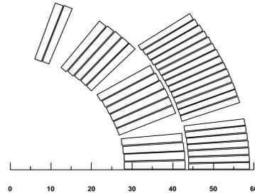
Figure 7: 6-block (38 turns) design (V6-3)
