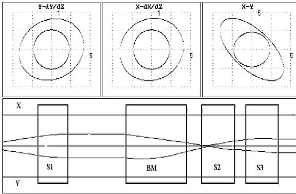
Figure 2. Phase ellipses and beam envelopes of SVAAP injection channel as given by LIDOS simulation code.
