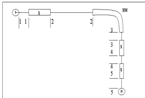
Figure 1. Schematic view of SVAAP focusing channel (S - solenoid lenses, BM - bending magnet, I - input point, O - output point, 1-1...5-5 – the distances (see table 3)).
