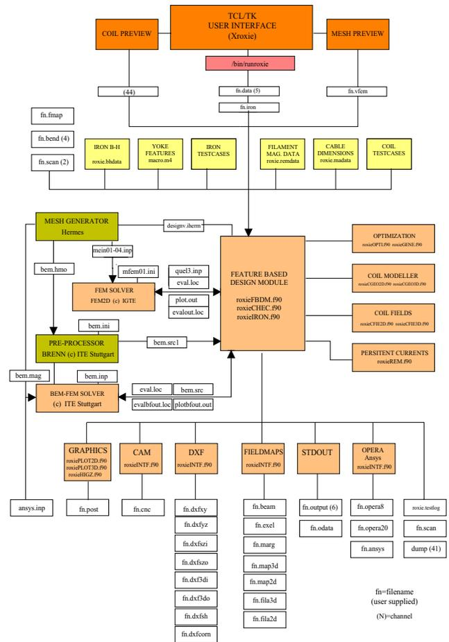
Figure 1: Structure of the ROXIE program featuring a TCL/TK user interface (top), and various interfaces to CAD-CAM (bottom). The interfacing to the finite-element packages is done by means of file transfer.
