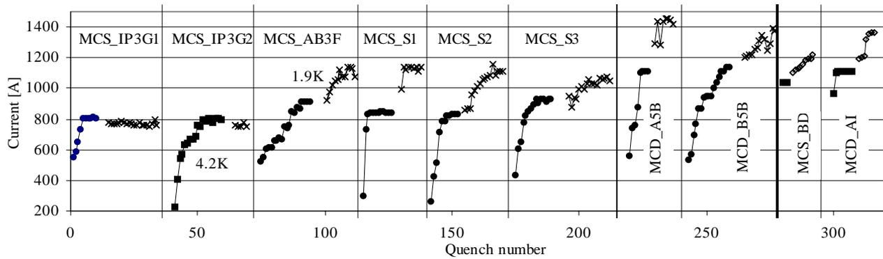
Figure 2: Training of sextupole and decapole models with double width coils. MCS\_BD and MCD\_AI are standard versions featuring 6 and 10 coils respectively. Wire used in MCS\_IP3G1&2 is unstable due too big sc-filaments.
