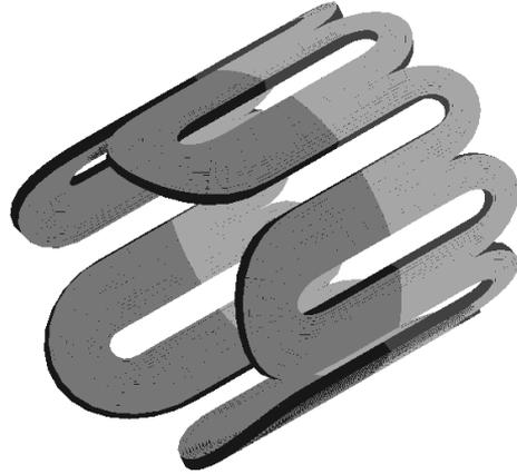
Figure 1: Principle of 5-coil and 10-coil decapole left and right respectively
