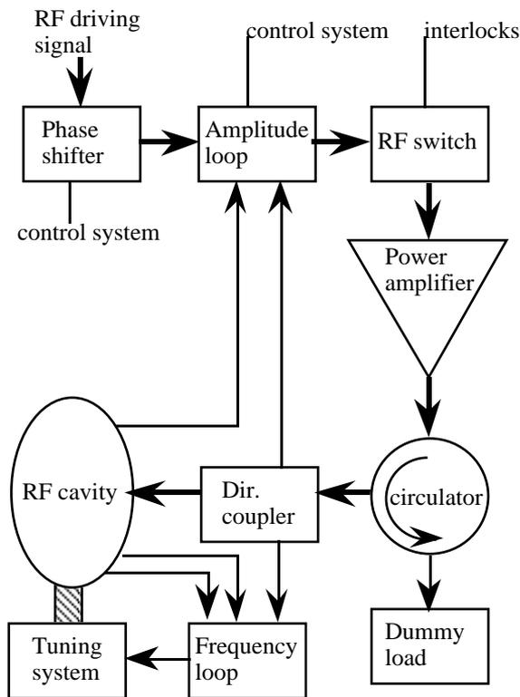
Figure 1: Block diagram of the booster RF system
