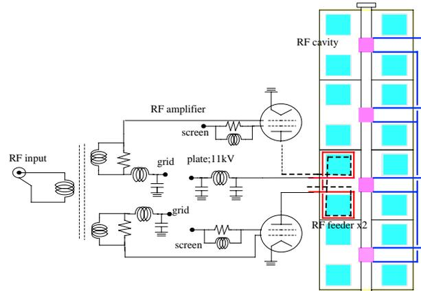
Figure 3: Schematic view of the cavity and amplifier.
