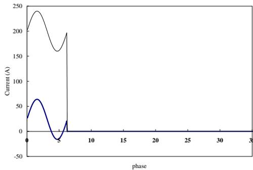
Figure 2: The required driving current for the barrier bucket. The thick and thin lines are for Q-values of 0.6 and 5, respectively. In the case of Q-value of 0.6, it is assumed that the resonant frequency is 1.5 MHz.
