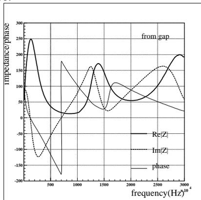
Figure 4: The gap impedance of the cavity.
