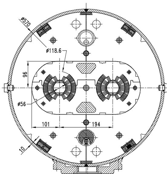
Fig.1 MBL Cross-section
