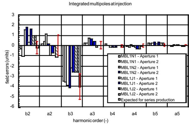
Fig.2 Values of the  $a_2, b_2$  to  $a_5, b_5$  harmonics measured at injection field for all long models.
