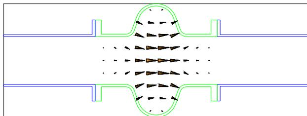
Figure 2a: Fundamental TM<sub>010</sub> mode electric field distribution.
