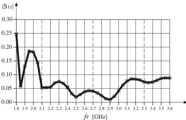
Fig. 7: Reflection coefficient of the transition.
