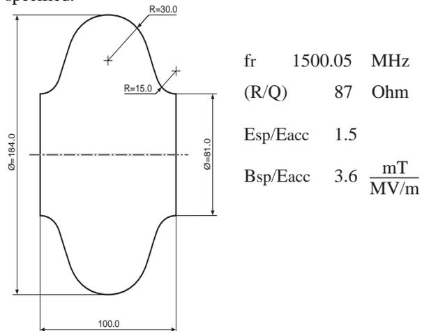
Figure 1: The cell geometry.
