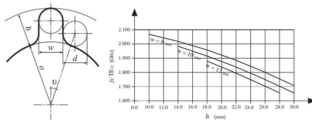
Figure 3: Dimensioning of the ridges.
