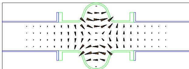
Figure 2c: Confined TM<sub>110</sub> mode electric field distribution.
