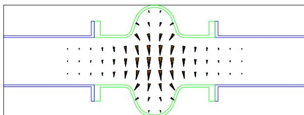
Figure 2b: Confined TE<sub>111</sub> mode electric field distribution.
