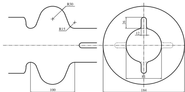
Figure 4: The cavity and the  $\phi$ -waveguides .
