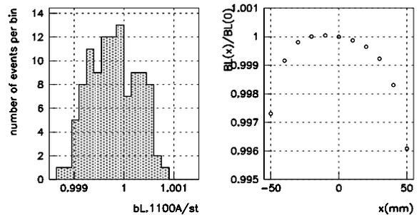
Figure 1 : Normalized integrated field histogram and an example of its transverse distribution for LER  $B_{arc}$
