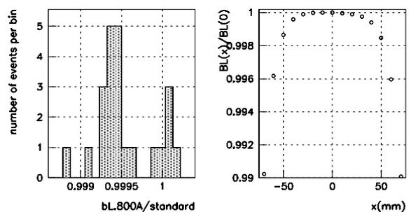
Figure 3 : Normalized integrated field histogram and an example of its transverse distribution for LER  $B_{lc}$
