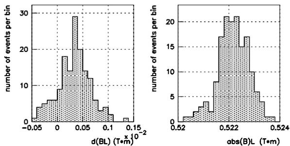
Figure 4 :  $\Delta[BL]$  and  $|B|L$  histograms of the wigglers
