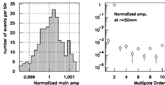
Figure 5 : Normalized integrated field gradient (left) and normalized multipole amplitudes plotted as a function of multipole order (right) for LER  $Q_{arc}$ .
