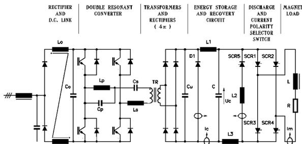
Figure 5: Circuit layout of DHPTT02 power converter.
