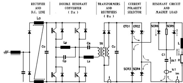
Figure 3: Circuit layout of DHPTT01 power converter.
