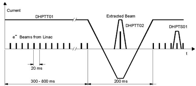
Figure 2: AR beam injection and extraction schemes.
