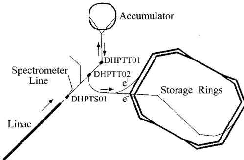
Figure 1: Beam transfer lines with three pulsed magnets.
