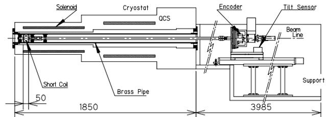
Figure 1: Magnetic field measurement system.
