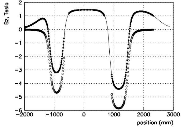
Figure 7:  $B_z$  distribution along the beam line. The open circle and the closed circle symbols correspond to the operations without and with the Belle solenoid, respectively. The solid line is the calculation.
