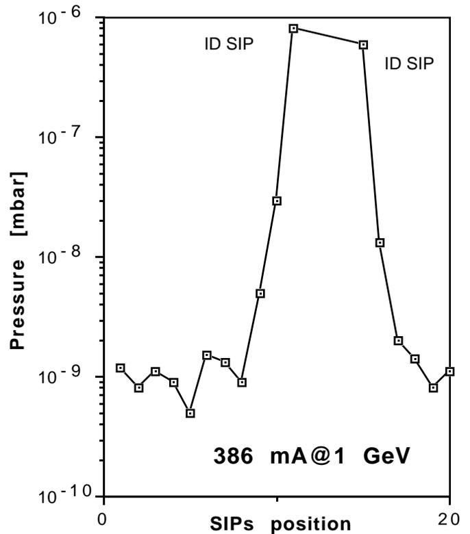
Figure 2: Pressure profile in the ID part of the II. vacuum sector
