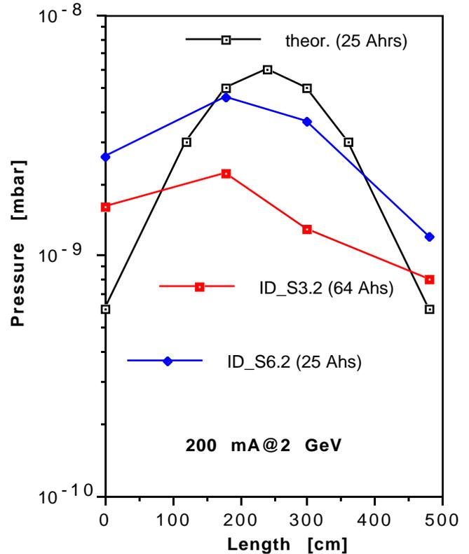
Figure 1: Theoretical and experimental pressure profiles with zero pumps in ID chambers
