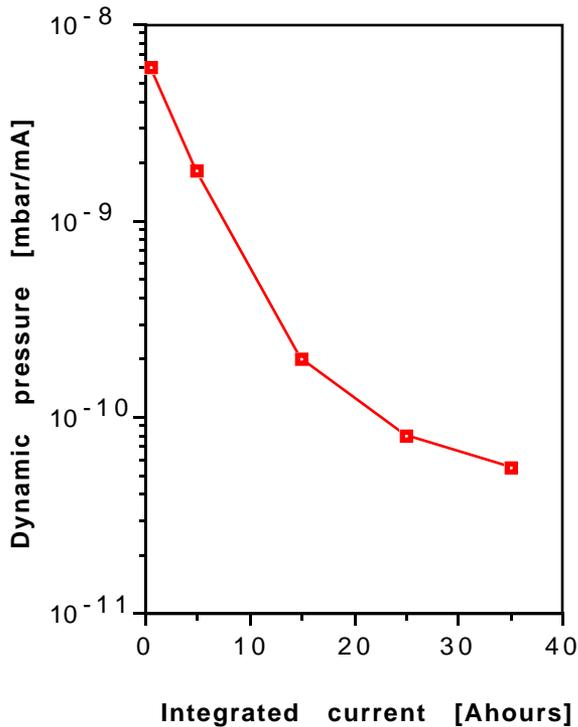
Figure 3: Dynamic pressure decrease (100 mA@2 GeV) in the pump free ID chamber during conditioning
