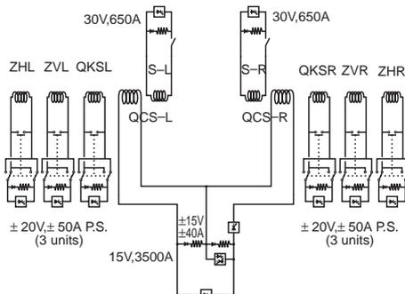
Figure 4: Electric circuit of the magnet system.
