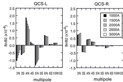
Figure 3: Harmonics of the quadrupoles at 40 mm radius
