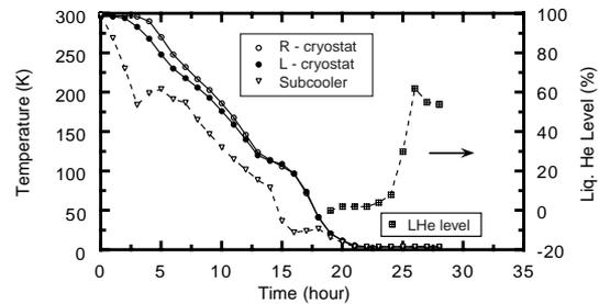
Figure 5: Cooldown curve of the magnet system.
