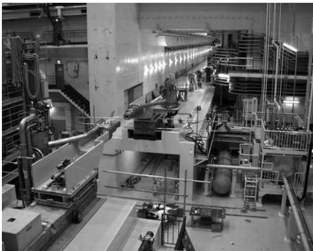
Figure 1: The final focus magnet system. The sub-cooler-cold-box unit is seen on the right side, from which two transferlines are running to the cryostat modules placed on two sides of the IP. The BELLE detector is rolled out towards the left in this photograph.
