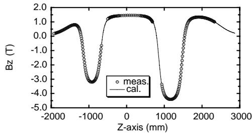
Figure 2:  $B_z$  distribution along the beam line when Belle detector solenoid ( $B_0 = 1.5\text{T}$ ) and two compensation solenoids are excited. The origin of the  $z$ -axis corresponds to the IP.
