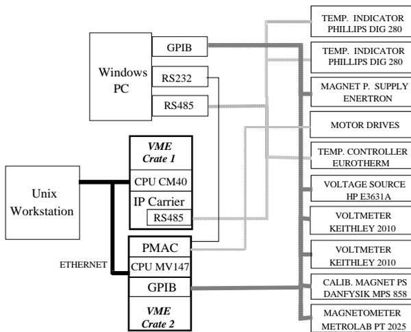
Figure 1. Block diagram of both hardware architectures used in the test bench.
