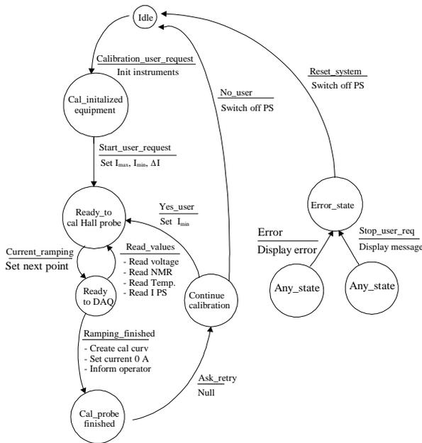
Figure 2. State Machine used to implement the calibration code with the EPICS Sequencer tool.
