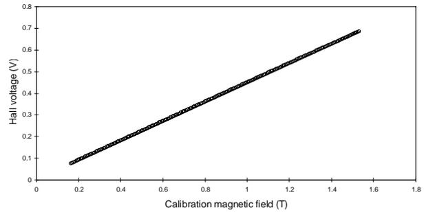
Figure 3. Calibration curve for the y Hall probe. The result is independent on the control system used.
