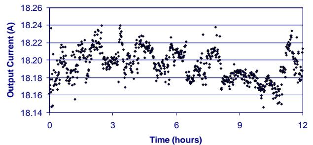
Figure 1. Long term stability of the prototype DC power supply.
