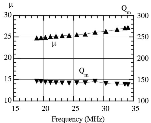
Figure 6: Measured  $\mu$  and  $Q_m$  for a ferrite
