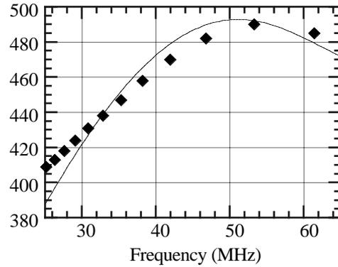
Figure 5: Resonance frequency and Q-value of the cavity without ferrite. Markes represent the experiment and the line is obtained by calculation.
