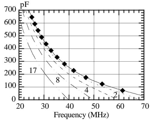
Figure 4: Tuning capacitance and frequency at resonance. Markers represent the experiment and solid line is obtained by calculation without ferrite. Dashed lines are by calculation with ferrite for various  $\mu$ , which are represented in figure.
