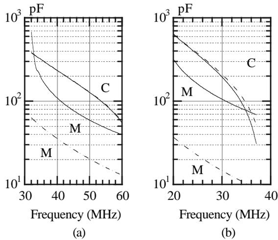
Figure 3: Tuning and impedance matching capacitance for  $\mu=2$  (a) and  $\mu=17$  (b). C means tuning and M matching capacitor. Solid lines are  $Q_m=20$  (a),  $Q_m=10$  (b) and dashed lines are  $Q_m=1000$  for both cases. Tuning capacitances are almost same in  $Q_m=20$  and  $Q_m=1000$  for  $\mu=2$
