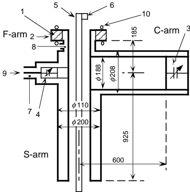
Figure 1: Schematic drawing of ferrite test cavity
