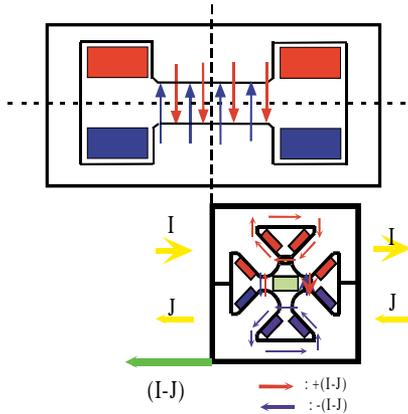
Fig. 3 Canceling of the common mode flux
