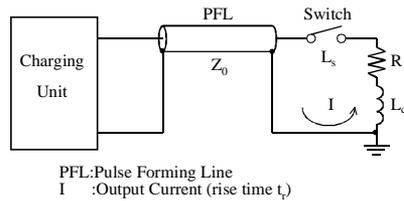
Figure 1. Basic pulse circuit for a kicker magnet system
