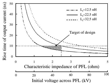
Figure 2. Dependence of rise time on impedance and total inductance
