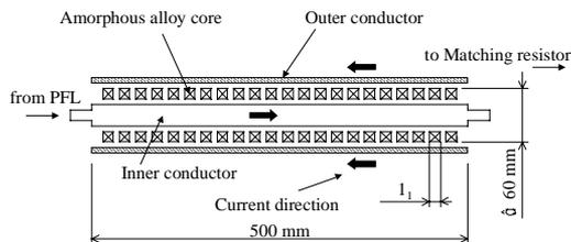
Figure 7. Schematic of the magnetic switch
