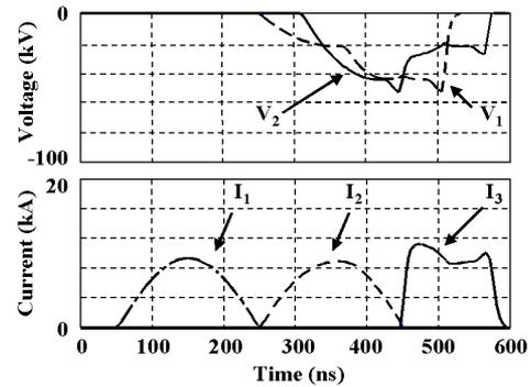
Figure 4. Simulated results of PFL pulse-charging circuit
