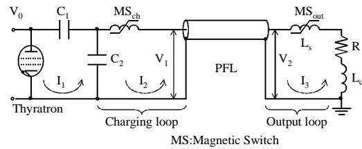
Figure 3. PFL pulse-charging circuit
