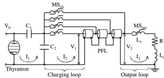
Figure 5. New type of PFL pulse-charging circuit
