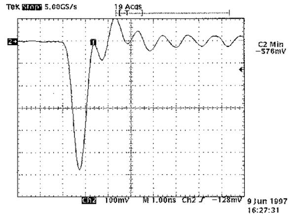
Figure 5. Gun current pulses, 1ns pulse width.
