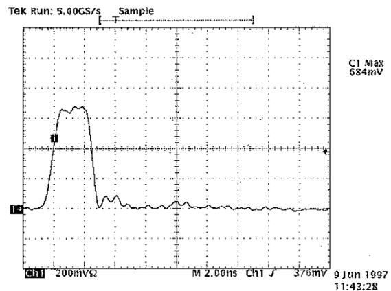
Figure 6. Gun Current Pulses, 4ns pulse width.
