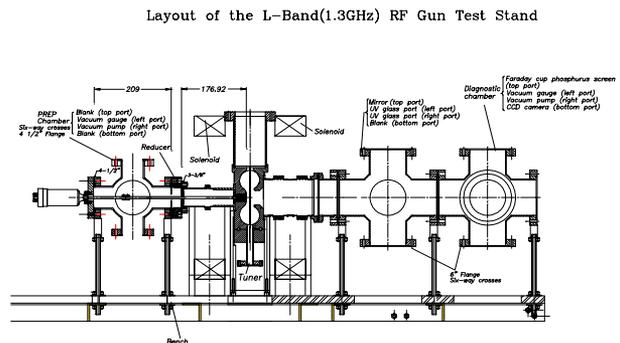
Figure 7: Layout of the L-band rf gun test stand.
