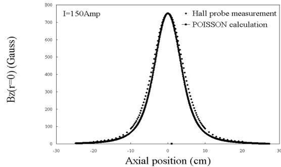
Figure 6: Longitudinal solenoid field profile on axis.
