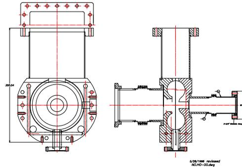
Figure 1: Assembly drawing of the gun cavity.
