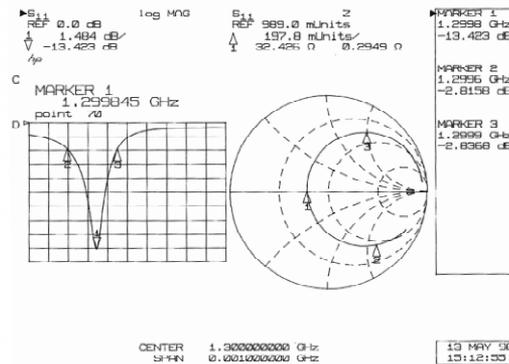
Figure 2: Measured reflection coefficient of gun cavity.
