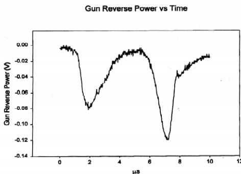
Figure 9: Reflected rf power from the gun. It shows that after the gun was filled, no reflection was observed.
