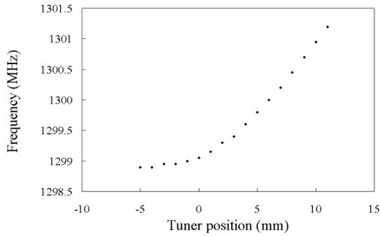
Figure 3: Measured resonant frequency to the tuner position.
