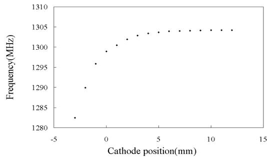
Figure 4: Measured resonant frequency to the cathode plug position.
