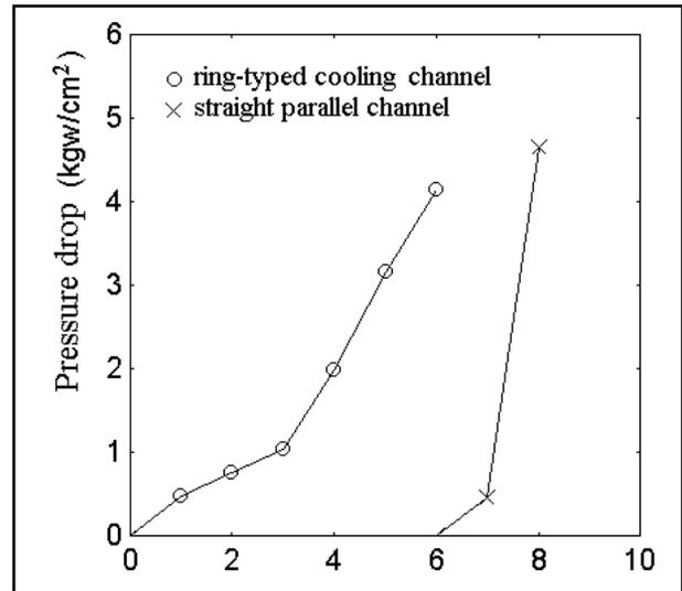
Fig. 3 Cumulated water pressure drop for ring-typed cooling channels(1-6) and straight parallel ones(7-8)
