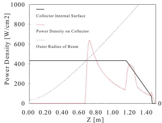
Figure 3: Simulation of Electron Beam Spread into the Collector
