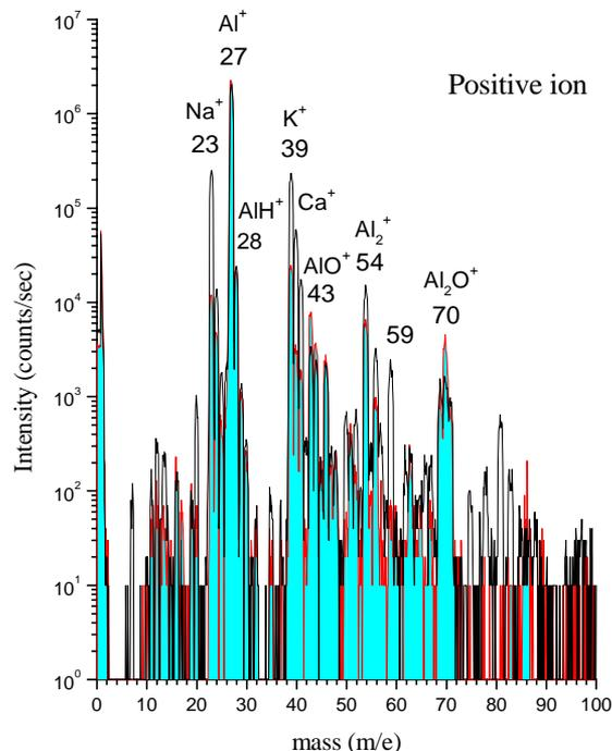
Figure 3. The positive secondary ion mass spectrum of Al alloy with (a) chemical cleaning only, (b) chemical cleaning followed by ozonized water rinsing (shaded area).
