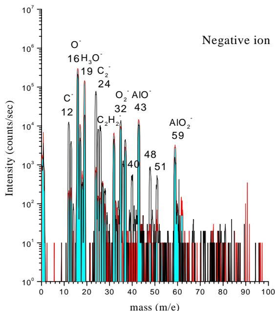
Figure 2. The negative secondary ion mass spectrum of Al alloy with (a) chemical cleaning only, (b) chemical cleaning followed by ozonized water rinsing (shaded area).
