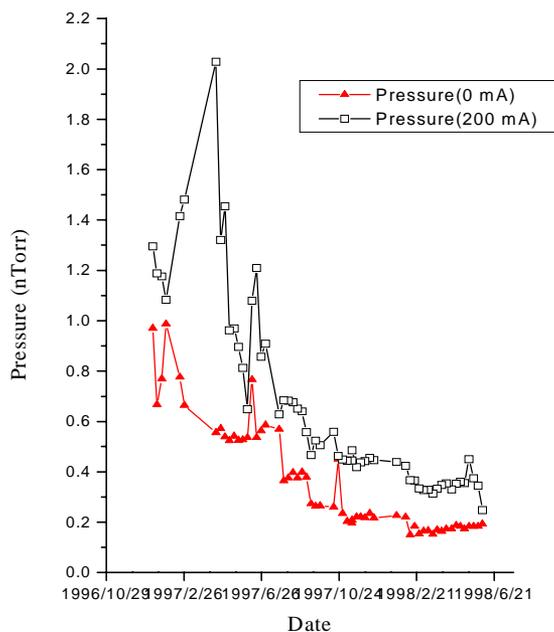
Figure 1. The average pressure of static vacuum and dynamic vacuum at 1.5 GeV, 200 mA in storage ring from the end of 1996 to 1998.
