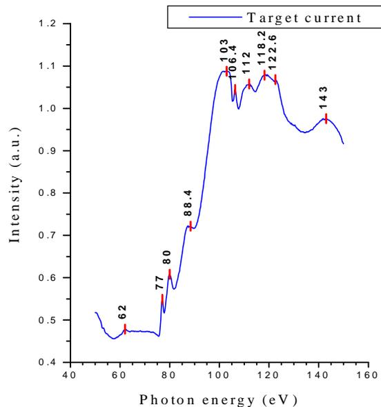
Figure 5. The target current measurement of Al alloy with variation of photon energy 50 ~150 eV.
