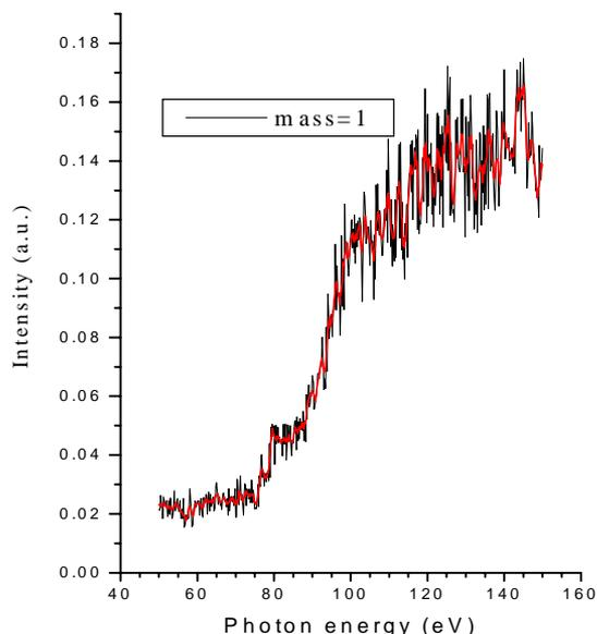
Figure 4. The photon stimulated ion desorption (PSID) spectra of mass=1 with variation of photon energy 50 ~150 eV.
