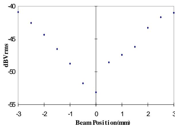
Figure 1: Beam position signal (dBVrms) versus beam position (mm).
