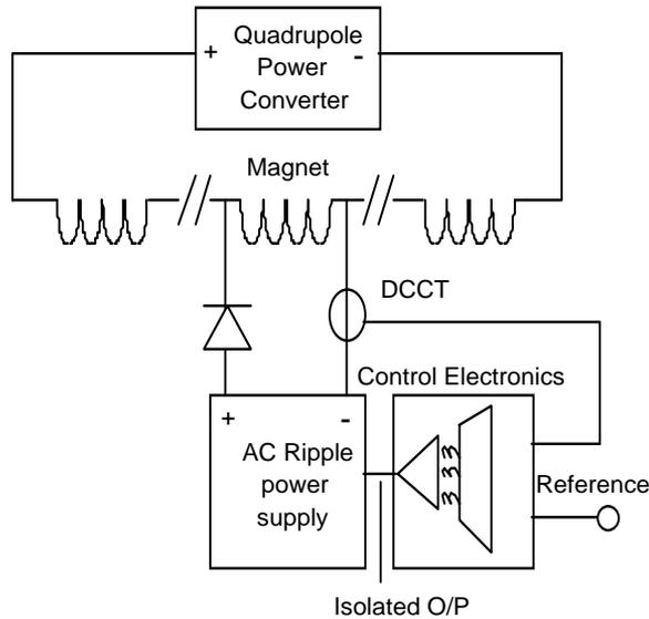
Figure 2: Superimposing a.c. ripple onto the d.c. excitation
