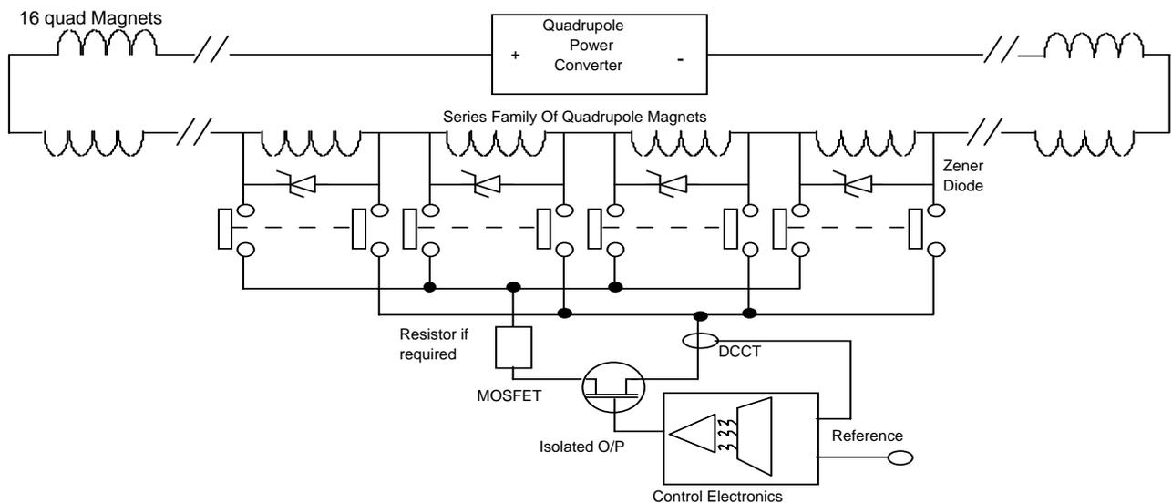
Figure 3: a.c. shunt design with common power and control electronics for four quadrupole magnets
