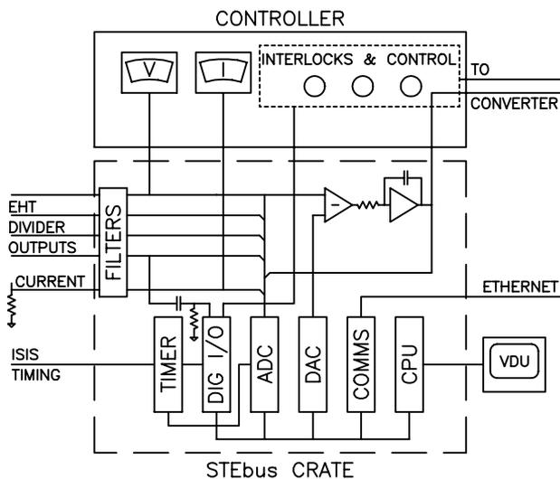
Fig. 3: Block diagram of Controller and CSS crate.
