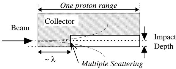
Figure 3: Longitudinal Collector Geometry
