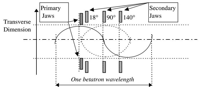
Figure 1: Schematic Of 1D Betatron System
