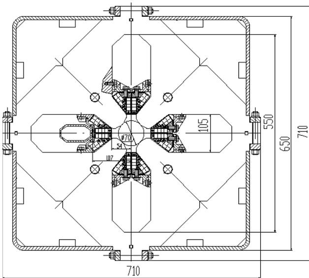
Fig. 3 Cross section of the magnet QN
