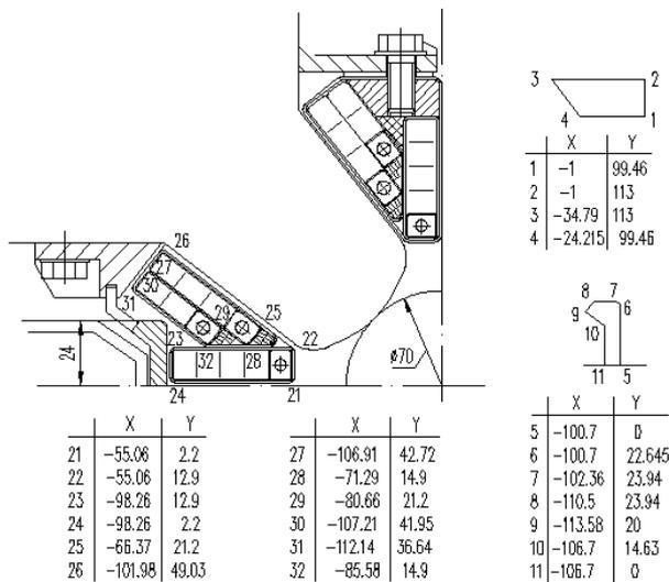
Fig.2. The results of the coil and shielding optimization
