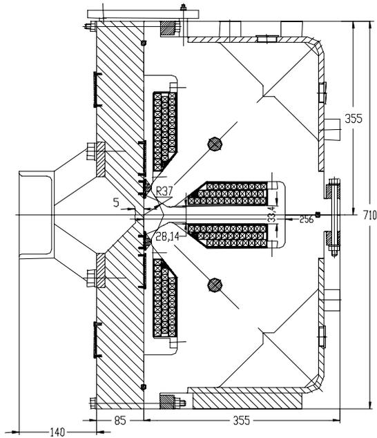
Figure 1: Cross section of magnet QM
