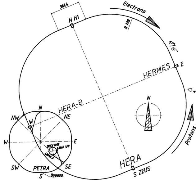
Figure 1: Layout of the electron proton collider HERA.
