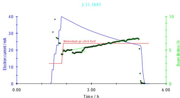
Figure 7: Electron operation with dipole pumps off.
