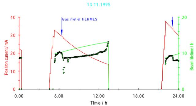
Figure 4: Change in  $e^+$  lifetime due to the helium target.
