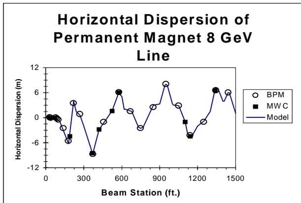
Fig. 7: comparison of the measured dispersion function of the 8 GeV line with the online computer model.
