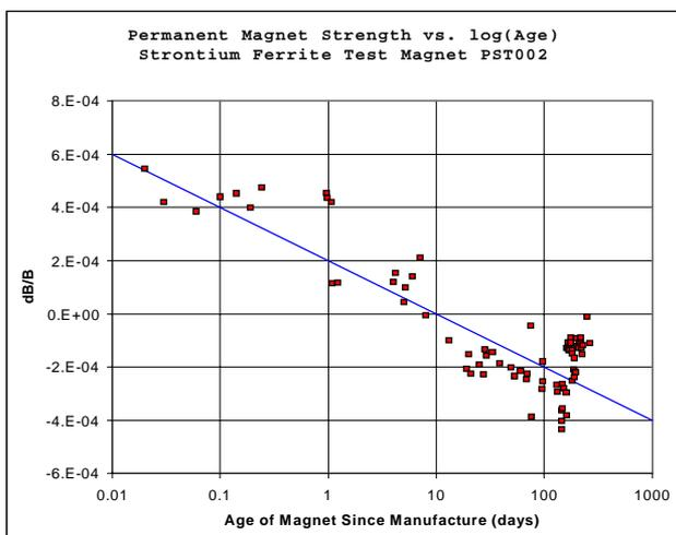
Figure 3: Time stability of a Strontium Ferrite test magnet measured for the Recycler Ring program. The magnet strength drops logarithmically with time, with a slope of  $\sim 2 \times 10^{-4}$  per decade.
