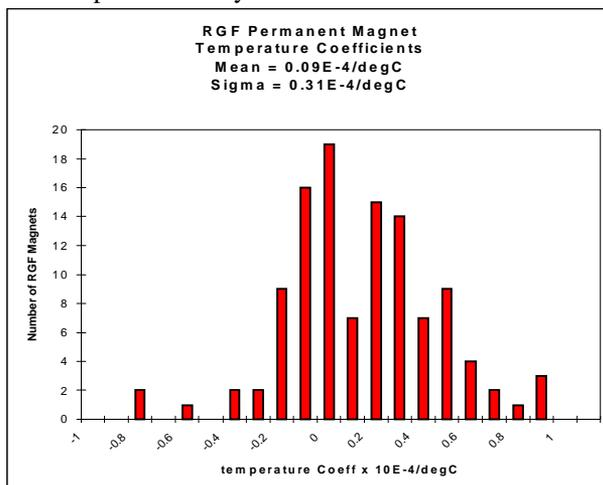
Figure 4: Temperature coefficients measured between  $0^{\circ}\text{C}$  and  $20^{\circ}\text{C}$  for Recycler RGF gradient dipoles.
