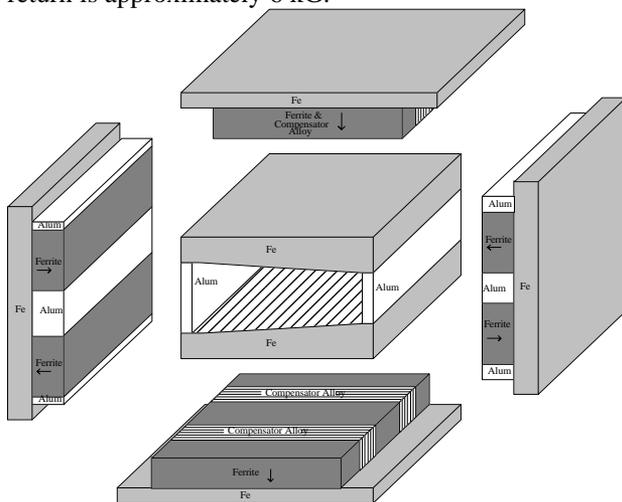
Figure 1: Cross-section of the 1.6 kG hybrid permanent magnet gradient dipole used in the 8 GeV line.
