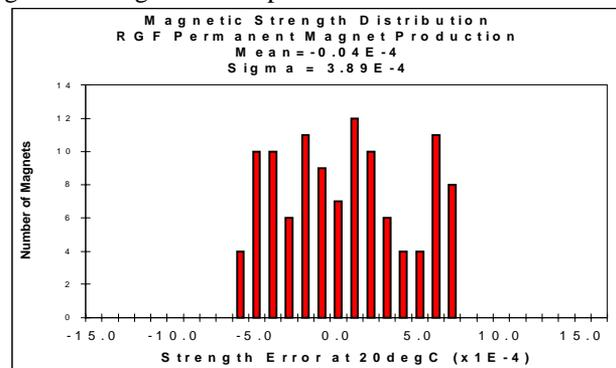
Figure 2: The strength distribution measured in production of Recycler RGF gradient dipoles. Magnets with strength errors outside of +/-6x10<sup>-4</sup> were adjusted by adding or subtracting a small amount of ferrite at the ends of the magnets.
