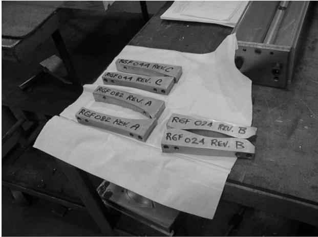
Figure 5: Customized end shims produced on a N/C mill to null out error multipoles on Recycler magnets.
