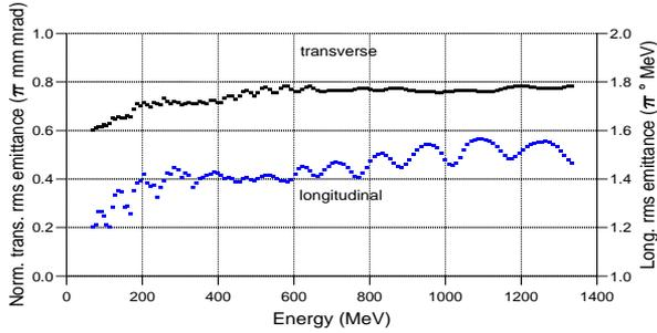
Figure 10: Rms emittances along the ESS linac for the mismatched case
