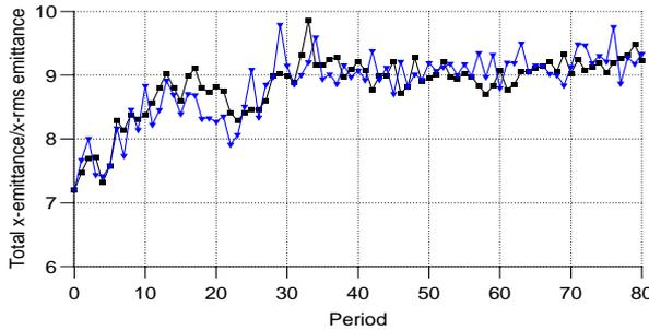
Figure 8: 99.9% total to rms emittance ratio for a matched (squares) and a high mode excited case (triangles). Please note the enlarged scale
