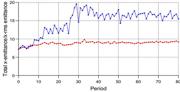
Figure 7: 99.9% total to rms emittance ratio for a matched (bottom) and a quadrupolar mode excited case (top)
