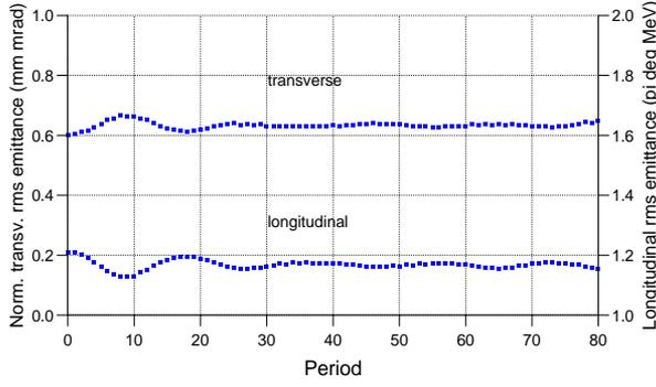
Figure 5: Rms emittances of the stable transferline
