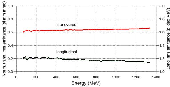
Figure 9: Rms emittances along the ESS linac for the matched case
