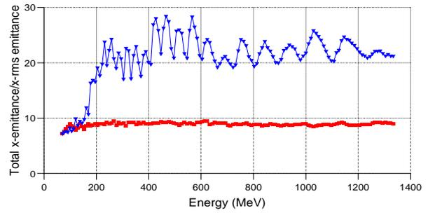
Figure 11: 99.9% total to rms emittance ratio in x-direction for a matched (bottom) and a mismatched case (top)
