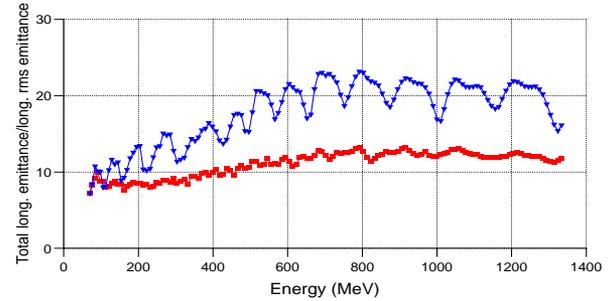
Figure 12: 99.9% total to rms emittance ratio in z-direction for a matched (bottom) and a mismatched case (top)
