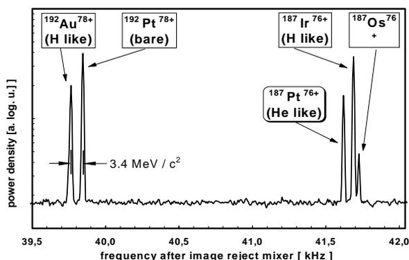
Figure 2: Zoomed part of a Schottky mass spectrum of electron cooled Au-fragments in the ESR. Additional lines are resolved from nearly 60 peaks seen in the original 100 kHz-spectrum. The published mass value for the  $^{187}\text{Pt}$ -nucleus could be improved essentially with respect to absolute value and relative error.
