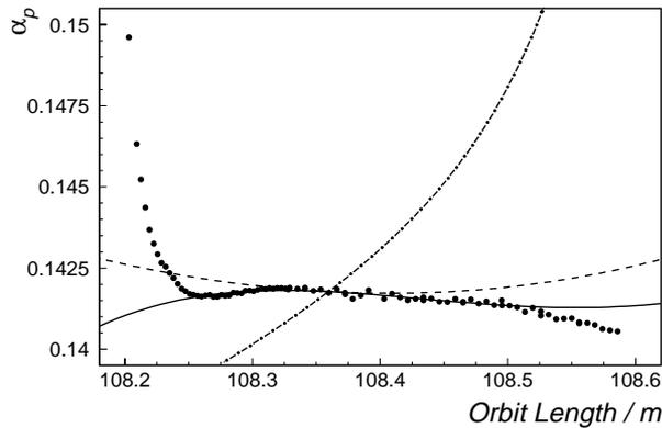
Figure 1: Experimentally determined  $\alpha_p$ -values (dots) for the ESR magnet setting used for SMS. Calculated curves for comparison take into account: dipoles including edge effects and quadrupoles (dash-dotted), addition of sextupoles (dashed), inclusion of pseudo-octupoles from quadrupole magnets (solid).
