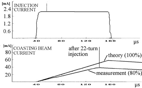
Figure 2: Multi-turn injection of  $1 \cdot 10^{11} \text{Ne}^{10+}$  -ions
