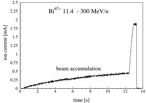
Figure 1: Beam accumulation by repeated multiturn injection with intermediate electron cooling.
