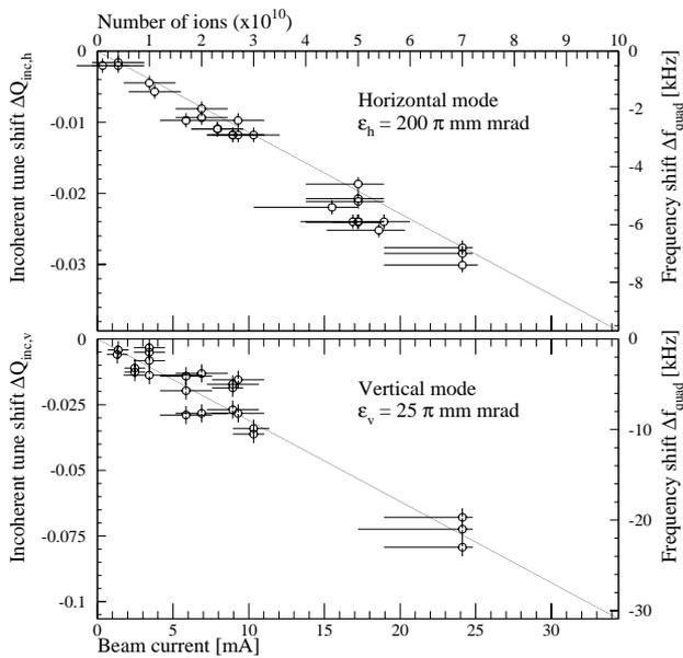
Figure 3: Incoherent tune-shift for the coasting  $\text{Ne}^{10+}$  beam at  $11.4 \text{MeV/u}$ .
