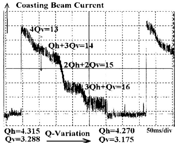
Figure 5: Beam losses at  $4^{\text{th}}$ -order resonances
