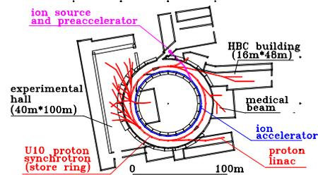
Figure 1. Layout of ITEP accelerator facility.
