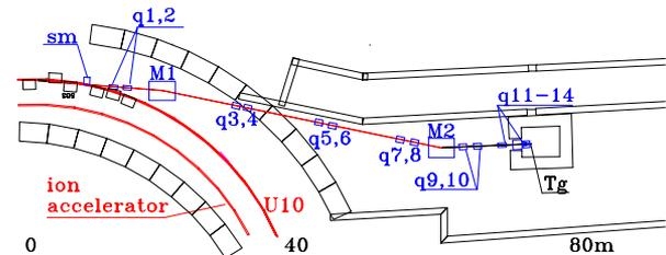
Figure 2. Layout of final beam transport channel for TWAC.
