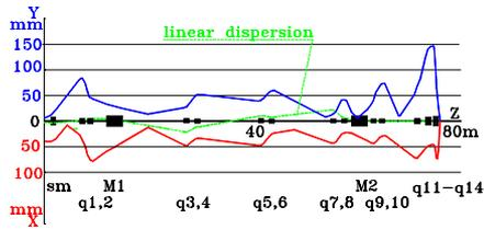
Figure 3. Optic scheme of final beam transport channel for TWAC.
