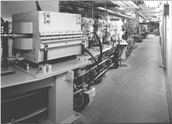
Fig. 2. Beam transport system at the NPTC
