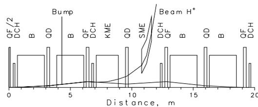
Figure 5: Beam ejection from the Booster.
