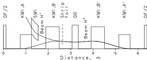
Figure 4: Beam injection into the Booster.
