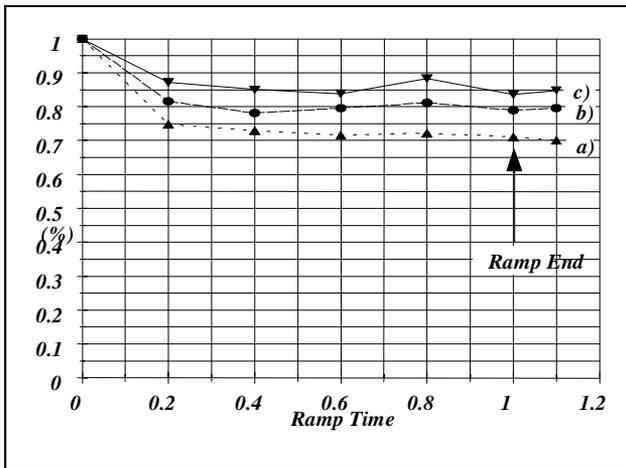
Figure 3: Beam transmission for one second ramps to 225 MeV for 3 values of RF acceleration voltage (see text).
