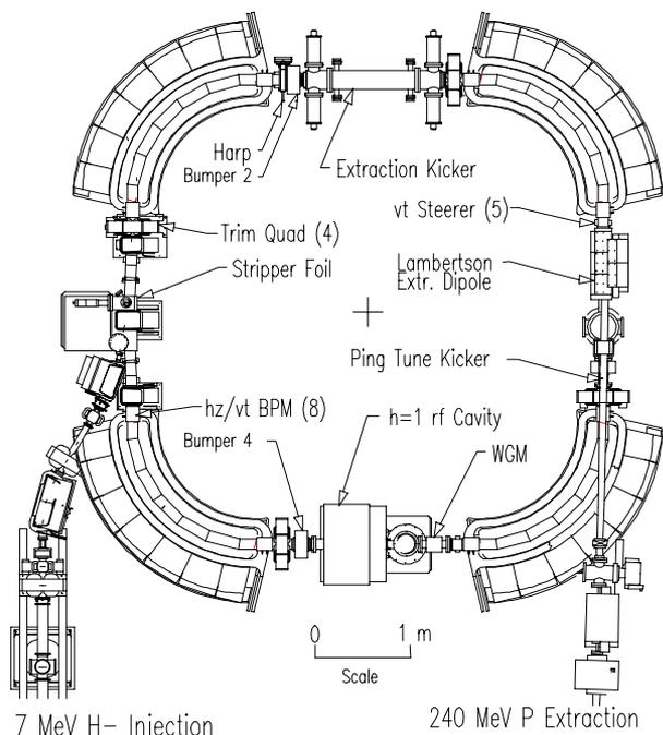
Figure 1: CIS Ring layout showing diagnostic elements.
