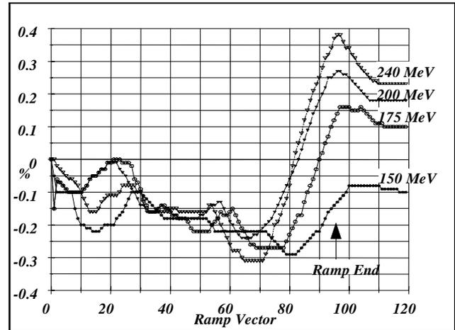
Figure 2: RF frequency corrections (%) as a function of ramp vector number for several flattop energies.
