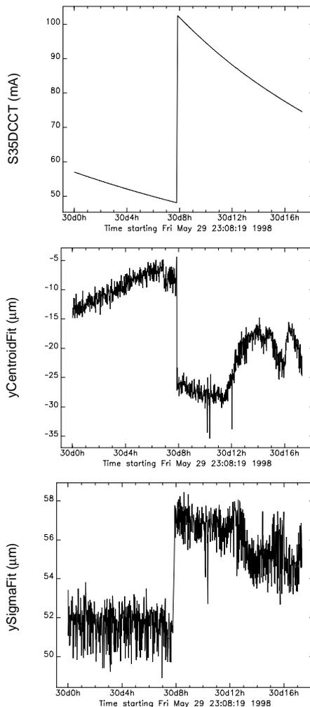
Figure 1: Data logging results for the stored beam current, beam centroid, and beam size for the vertical plane, respectively, from top to bottom.
