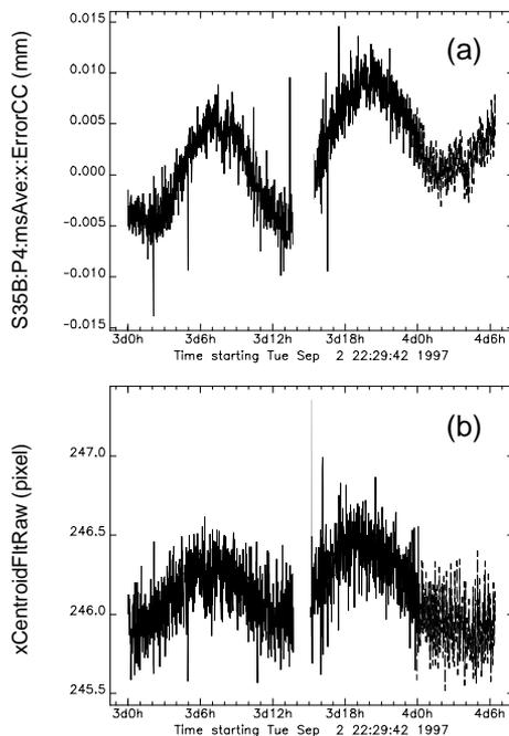
Figure 3: Comparison of the beam centroid position from the nearby rf BPM (a) and the pinhole camera image (b) over  $\sim 30$ -hour period. The 10- $\mu\text{m}$  modulation of horizontal beam position over 24 hours is attributed to the moon's gravitational effects on the effective beam orbit circumference.
