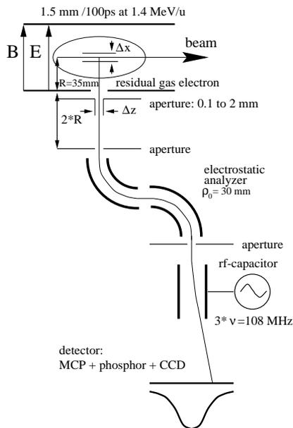
Figure 3: Schematic sketch of the designed device for the bunch length measurement.
