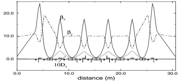
Figure 4: Plot of another five bend achromat FBA2 lattice. Plots of  $\beta_x$ ,  $\beta_y$ , and  $10 \times D_x$  are shown. The upward and downward lines are focusing and defocusing sextupoles.
