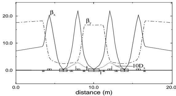
Figure 2: Plot of the triple bend achromat lattice. Plots of  $\beta_x$ ,  $\beta_y$ , and  $10 \times D_x$  are shown. The elements represented as single line are sextupoles, where the upward and downward lines correspond to focusing and defocusing sextupoles respectively.
