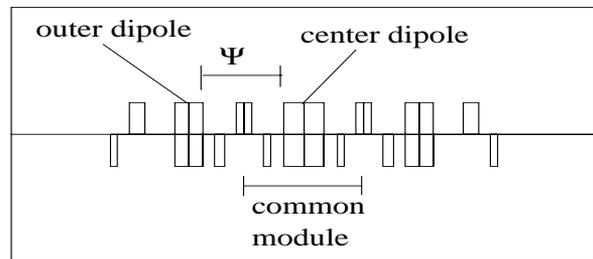
Figure 1: Layout of a triple bend lattice. Note that the center dipole is  $3^{1/3}$  times longer than the outer dipole. Common module and  $\Psi$  the phase advance are marked. For the design of a nBA with  $n \geq 4$ , additional constraints  $\alpha_x = 0$ ,  $\alpha_y = 0$ , and  $D'_x = 0$  are imposed at the both ends of common module. Symmetric common modules can be inserted into the lattice for a minimum emittance nBA.
