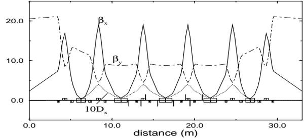
Figure 3: Plot of a five bend achromat FBA1 lattice. Plots of  $\beta_x$ ,  $\beta_y$ , and  $10 \times D_x$  are shown. The upward and downward lines are focusing and defocusing sextupoles.
