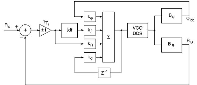
Figure 2. State variable feedback.  $B_R$  and  $B_\phi$  are beam transfer functions. There are four states, including an integral of the radial error and a delay compensator. At transition the sign of the radial feedback is changed.
