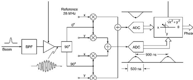
Figure 3. The bunch-by-bunch phase measurement circuit. The I/Q components of the response of the Bessel filter ( $Q=10$ ) are demodulated with the components of the reference signal at 28 MHz. Digital rectangular-to-polar conversion supplies the phase and magnitude.
