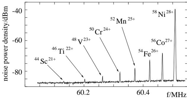
Figure 4: A  $^{58}\text{Ni}$  primary beam and fragments with similar magnetic rigidity stored in the ESR during isochronous operation. The relative differences in mass-to-charge ratio between two adjacent peaks in this spectrum is  $1 \dots 2 \cdot 10^{-3}$ .
