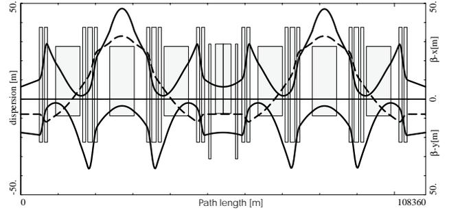
Figure 1: ESR operation mode with low transition energy. Dispersion (dashed line) and betatron functions (solid lines) are given. The lattice structure is sketched for orientation purpose.
