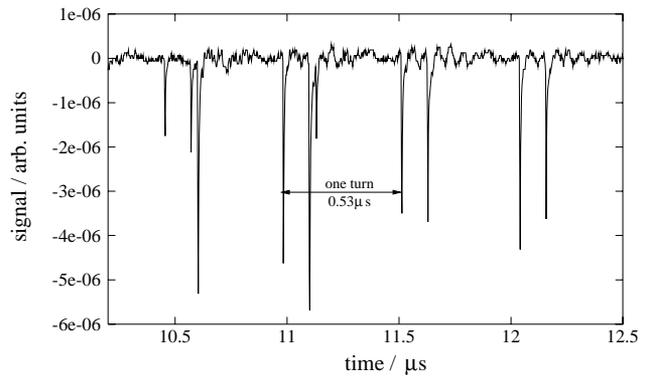
Figure 6: Trace of the analogous detector signal induced by three ions circulating in the ESR. Two of these ions are observed four times while the third one disappears in between. For mass measurements the timing properties of the signal will be improved substantially. We expect to resolve signals of ions separated by only a few ns.
