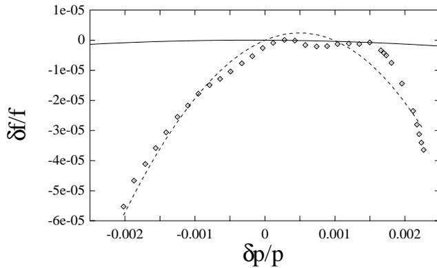
Figure 2: Comparison of measured frequencies (data points) to calculated ones: The dashed line reflects the result from a MIRKO-calculation carried out as described above, using a linear dependence of  $\gamma_t$  on the momentum. The solid curve shows the result calculated with an improved sextupole setting (see 4).
