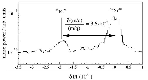
Figure 5: Part of a frequency spectrum recorded in the isochronous mode of operation of the ESR. The two observed species differ in mass-to-charge ratio by only  $\approx 3.6 \times 10^{-5}$ .
