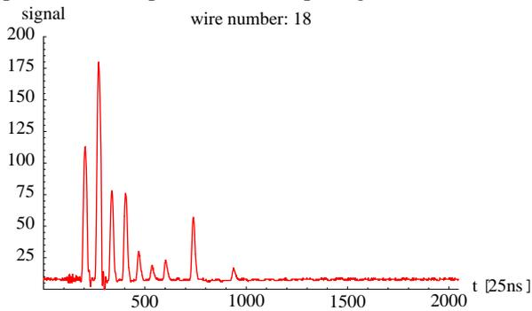
Fig. 2: Signal on a single wire. Each peak corresponds to one turn in the accelerator.
