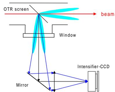
Fig.5: Matching monitor set-up in the SPS
