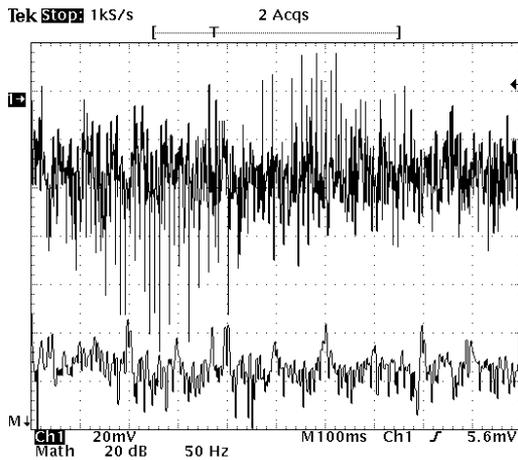
Figure 7: Example of worst case beam vibrations in the vertical plane, and corresponding FFT spectrum.
