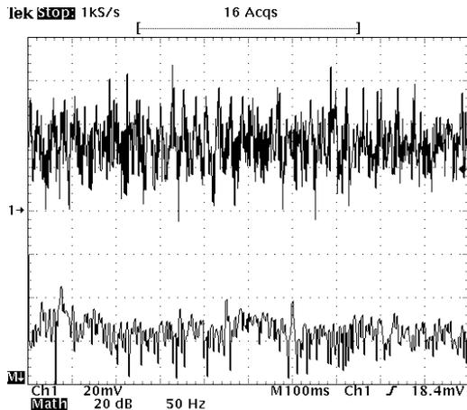
Figure 8: Example of beam vibrations in the vertical plane, and corresponding FFT spectrum.
