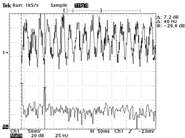
Figure 3: Detector signal from 40 Hz, 50  $\mu\text{m}$  beam excitation, and corresponding FFT spectrum.
