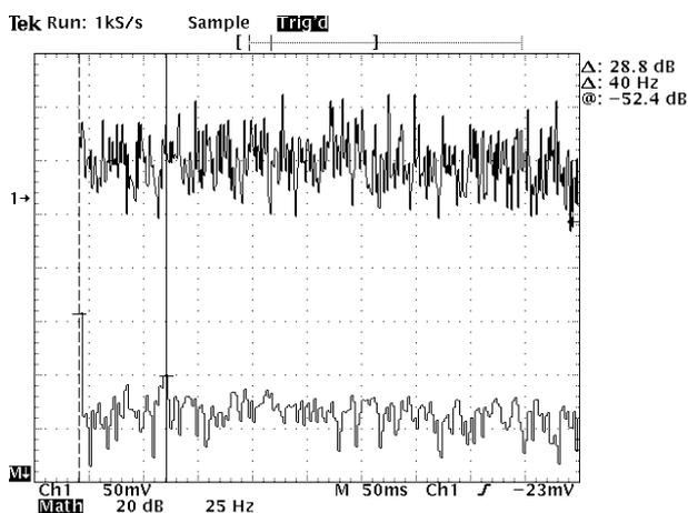
Figure 4: Detector signal from 40 Hz, 5  $\mu\text{m}$  beam excitation, and corresponding FFT spectrum.
