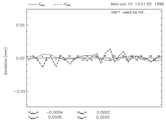
Figure 2: Closed orbit with 5  $\mu\text{m}$  DC beam excitation.
