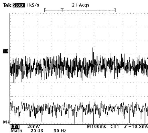
Figure 5: Detector signal using HeNe laser as light source, and corresponding FFT spectrum.
