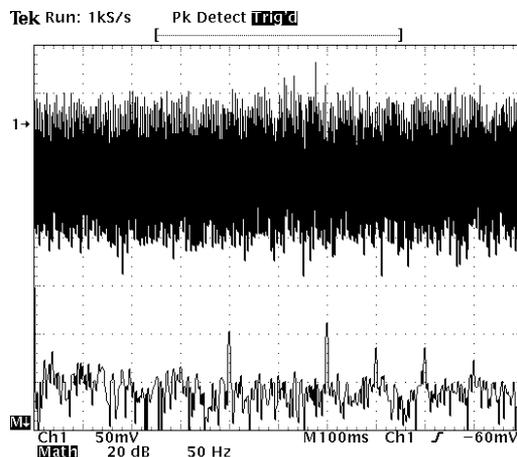
Figure 6: Example of beam vibrations in the horizontal plane, and corresponding FFT spectrum.
