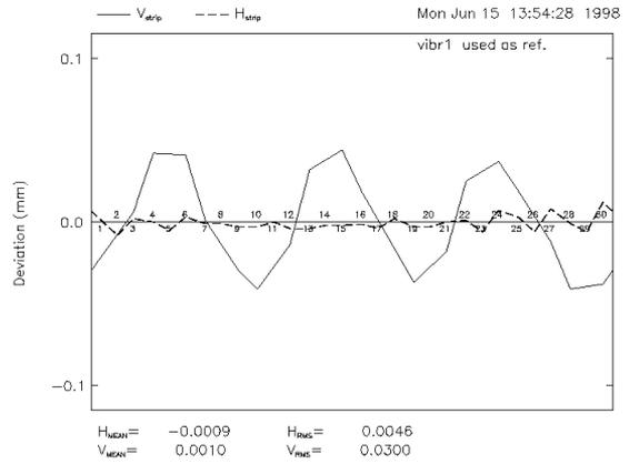
Figure 1: Closed orbit with 50  $\mu\text{m}$  DC beam excitation.
