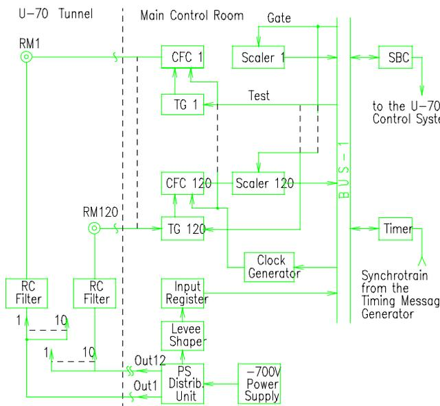
Fig. 3. A simplified block diagram of the Beam Loss Monitoring System
