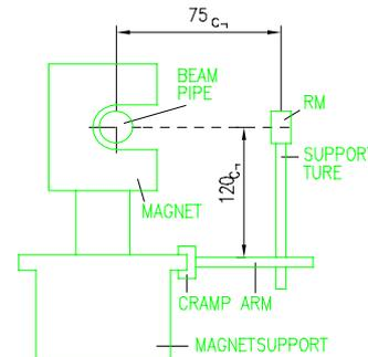
Such a mounting ensures maximum monitor sensitivity to beam losses and uniform geometry with respect to the closed orbit; also, it does not block access to the magnet and the beam pipe. Magnetic materials are not used in the detector, so the magnetic field force does not act on the detector body. The monitor is attached to the support duralumin tube. The lower part of this tube is clamped in a horizontal steel arm, and the last one is attached to the magnet support by a cramp.
