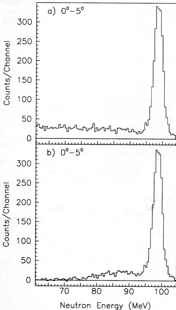
Figure 4: (a) Reconstructed energy spectrum of incoming neutrons, using a proton spectrum in the angular range  $0-5^\circ$ , obtained with a  $\text{CH}_2$  target, and subtracting the contribution from the  $^{12}\text{C}(n,p)^{12}\text{B}$  reaction. (b) The same spectrum as in (a) using TOF-gating.
