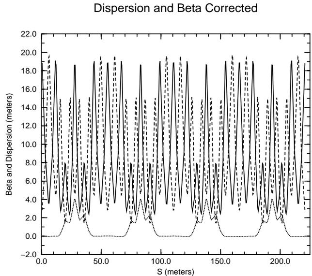
Figure 4: Same as above but with dispersion and beta corrected.
