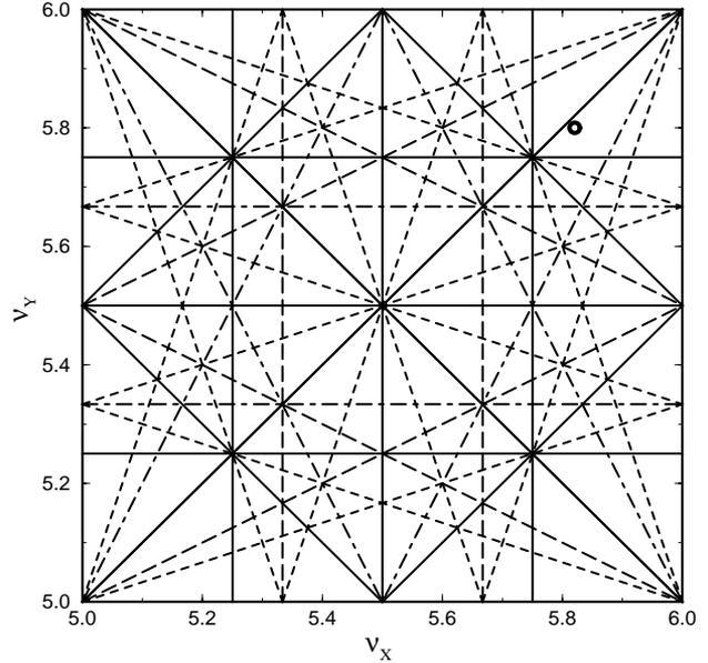
Figure 1: Accumulator Tune Chart. The circle shows the working point. Solid and short-dashed lines indicate second and fourth-order resonances; long-dashed and dot-dashed lines indicate third-order.
