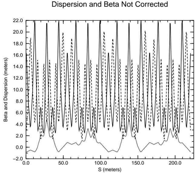
Figure 3: Dispersion and Beta distortion due to quadrupole errors with tunes near 6. Solid and dashed curves indicate horizontal and vertical beta functions respectively; dotted curve indicates dispersion.
